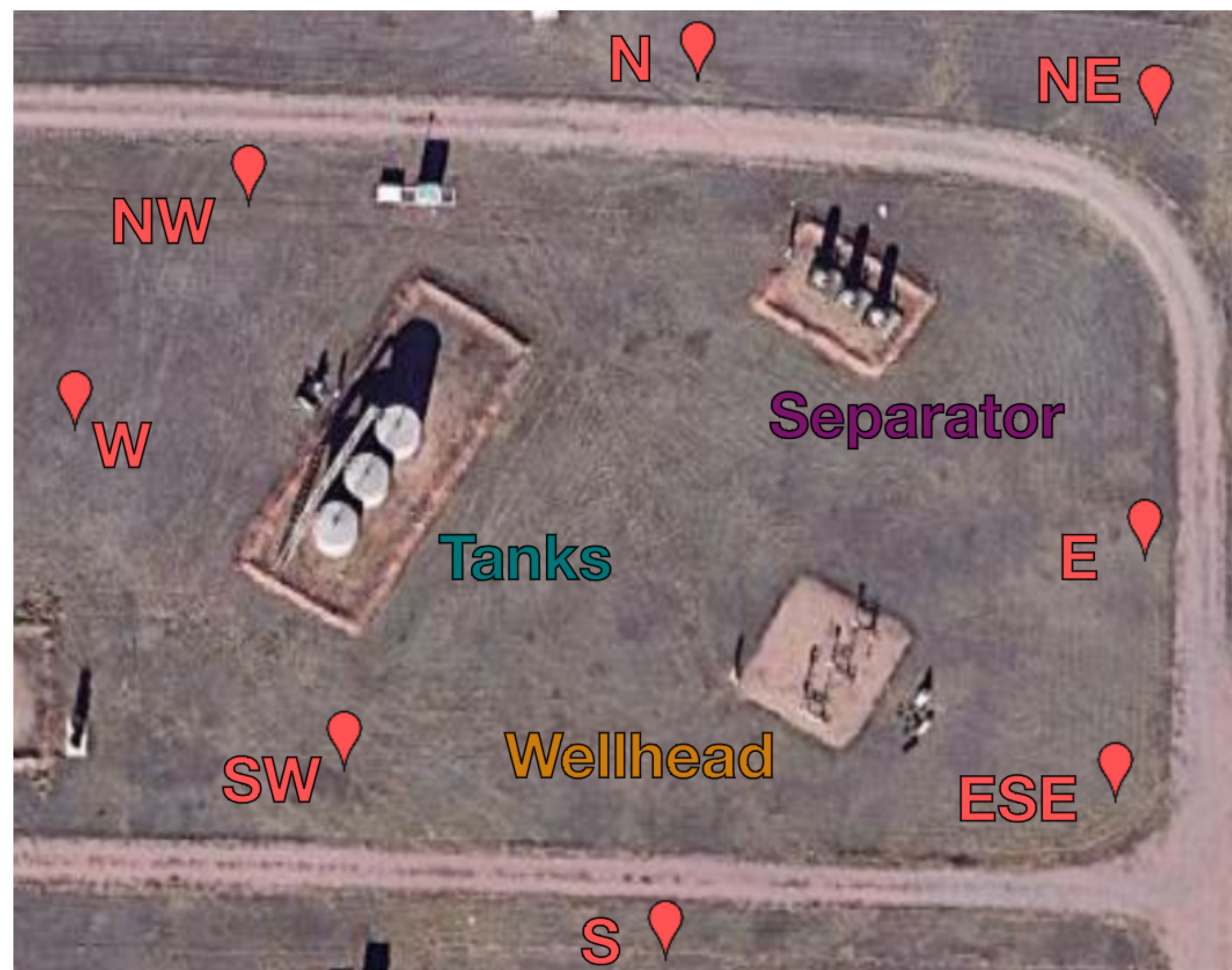
Figure 1: Configuration of METEC experiment
