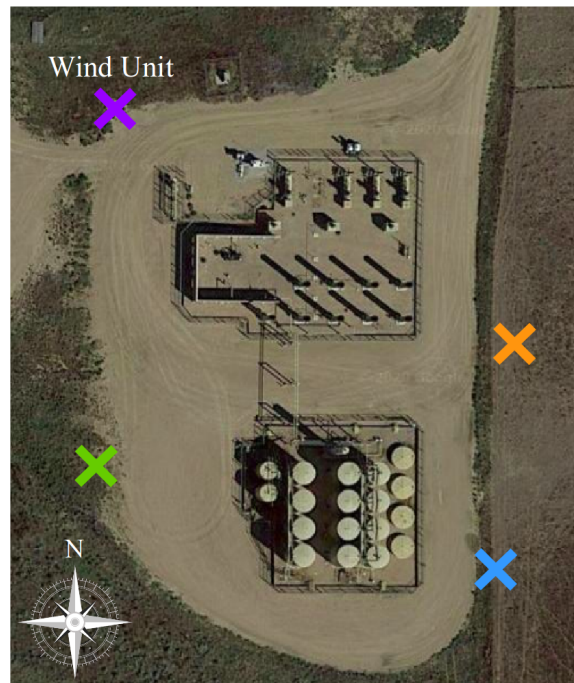
Figure 2: Geometry of Site A. Locations of the four Canary units are marked with X's. The northwest unit is the only unit on site that measures wind.
