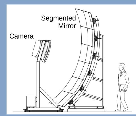
• Each camera has 440 PMTs and 10 MHz acquisition rate.
